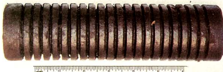
Figure 1. Blowdown sample filter plugged with iron oxide (~ 50 grams)
